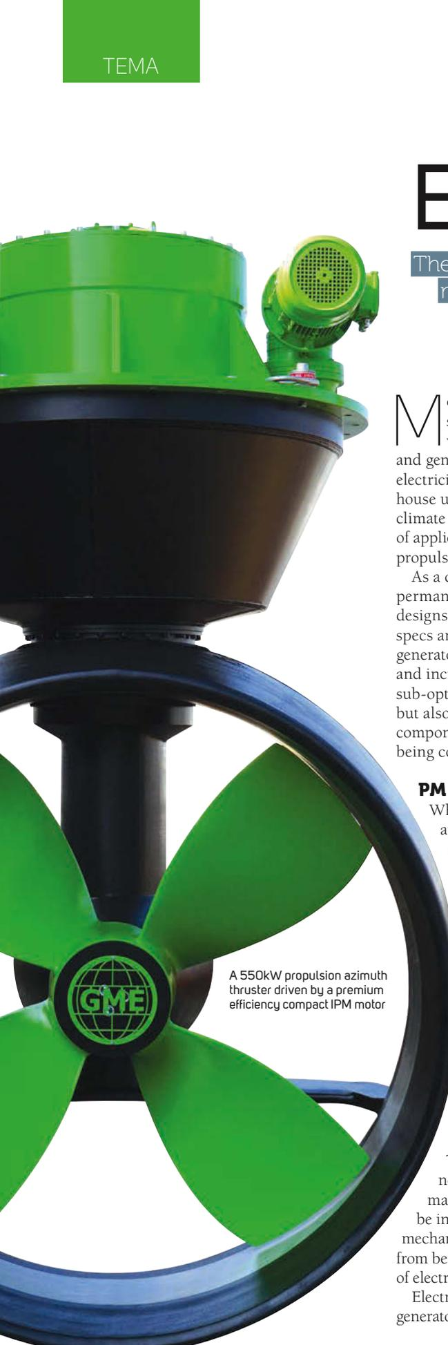
A 550kW propulsion azimuth thruster driven by a premium efficiency compact IPM motor
